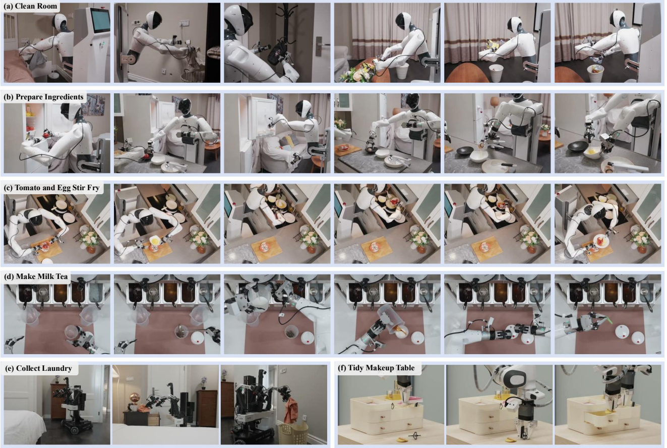
Fig. 3: Representative physical-robot evaluation tasks. (a) Clean Room requires collecting two dirty garments, placing them in a laundry basket, hanging a handbag, handing a blanket to a person, and disposing of table trash. (b) Prepare Ingredients requires retrieving a tomato and an egg, then cracking and stirring the egg while returning the tools. (c) Tomato and Egg Stir Fry requires chopping and transferring the tomatoes, cooking and seasoning the ingredients, plating the dish, and returning the cookware and utensils. (d) Make Milk Tea requires adding toppings, pouring milk and tea, sealing the cup, and inserting a straw. (e) Collect Laundry requires transferring a T-shirt from the bedside table to a laundry basket. (f) Tidy Makeup Table comprises three separately scored instruction-following groups that require different object selections and action sequences from matched visual states.
